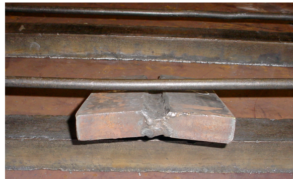
U-Shaped groove by carbon arcing
